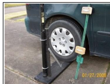
*Two pole supports. One is held up by the car and the other one is driven into the ground and has U clamps that support the telescoping pole.*
