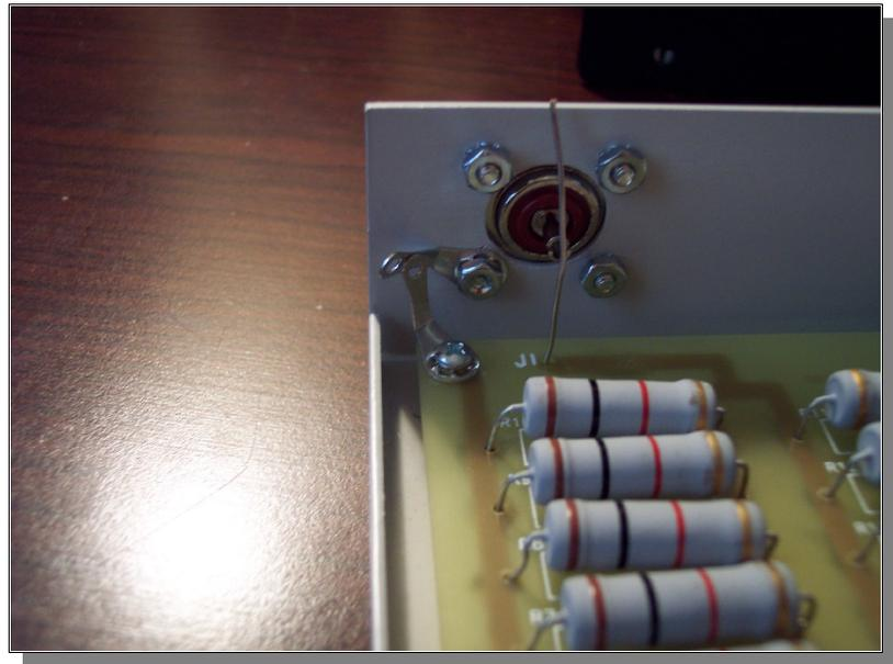
Once I had it all finished, I hooked up the Ohm Meter and checked my work. The display bounces between 50 and 51 Ohms as shown in the photo. On another Ohm meter it's exactly 50 Ohms, which is what Ohm's Law says it ought to be.
