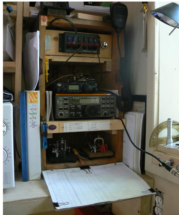
In the middle section, I have my K2 for use on CW and the Yaesu FT-817-ND for use on SSB and 6m. The J-38 key on top of the '817 is used for CW on 6m if the need arises. I have to use an Elecraft T1 autotuner with the '817 and I normally keep it on the small shelf above the cabinet. The K2 is "optimized" for low current usage (see this issues article for more details on this).
